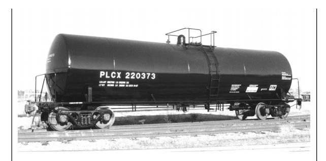
**PLCX 220373** is a 20,507 gallon insulated coiled tank car. Built by Trinity Industries, Longview, Texas in November 1987. Trinity File # 8724. AAR car type code T105. External length 48'11".
