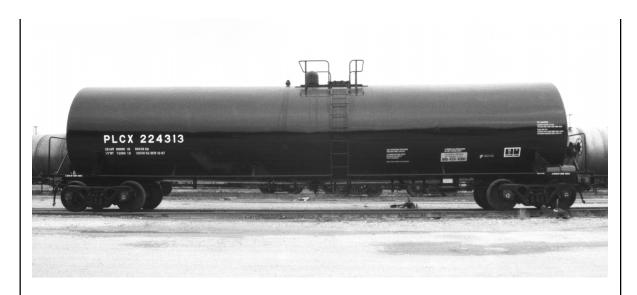
**PLCX 224313** is a 23,711 gallon insulated coiled tank car. Built by Trinity Industries in December 1987 (File # 8723). AAR car type code T106. External length 55'5".
