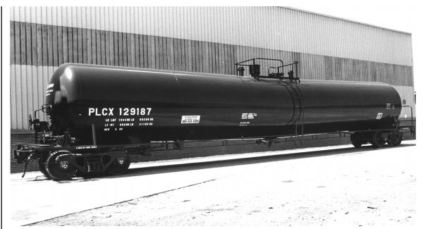
**PLCX 129187** is another non-insulated un-coiled tank car built under builder's reference # 6589 by Union Tank Car. This one was built in May 1989. Capacity is 30,010 gallons. DOT class 111A100W1. Non-insulated un-coiled. AAR car type code T108. External length 69'0".
