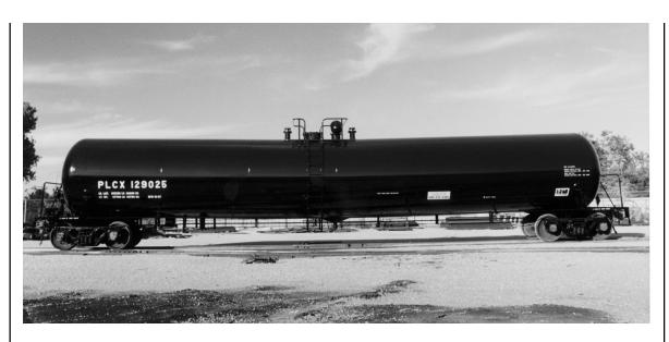
**PLCX 129025** is a non-insulated tank without coils. This is the type of tank that usually carries alcohol, methanol and related products. This has a 29,815 gallon capacity. It was built in October 1987 by Trinity Industries (File # 8725). DOT class 111A100W1. AAR car type code T108. External length 67'11".
