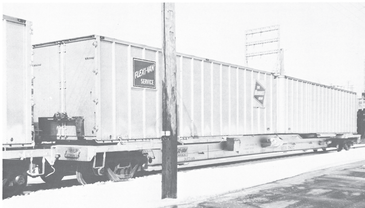
MILW 58017. A Mark I flat car carrying MM4047 a 36-foot closed van. (Milwaukee Road photo; R. Yaremko Collection)
