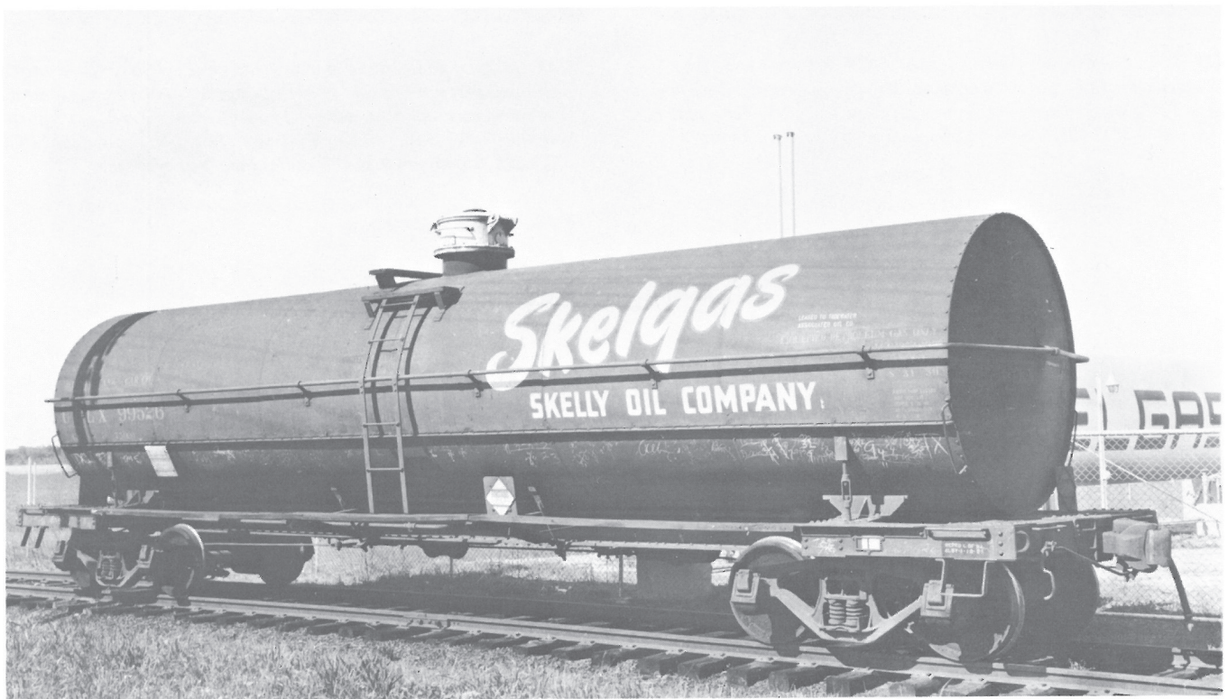
UTLX 99526 c.1954 was being leased to Tidewater Associated Oil Co. (see the stencil just to the right of the large "Skelgas" — stencilled lessee marks usually "override" any logos that may be present). This LPG car was built in August 1939. Note not only the small side platform but also the platform atop the tank next to the controls housing. Black tank with GOLD lettering (not yellow — ask Union Tank Car). The Skelgas etc. is white.
